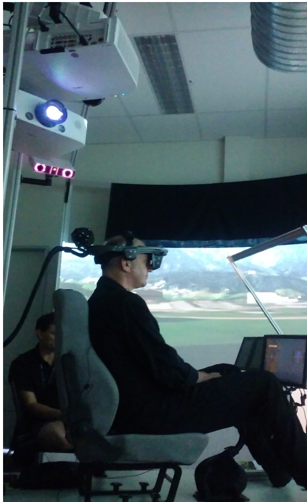
Figure 7. : An example of the simulator setup. The pilot has the head piece attached which displays the HUD information over the simulated environment. In front of the pilot are the electronic map and a multi-function display, which indicated altitude, ground speed, collective power and helicopter roll.
